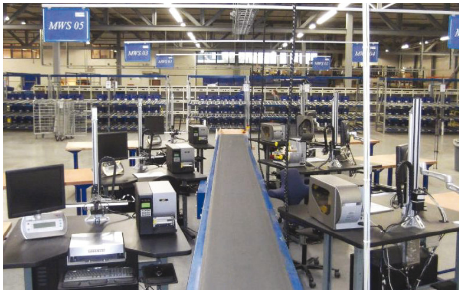
ID Mail's manual mail workstations allow Sandd to efficiently process small batch and non-machinable mail
